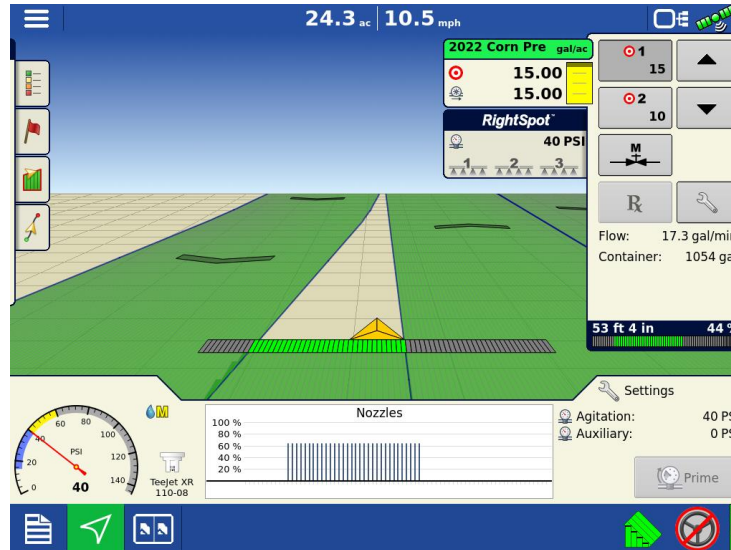
Figure 2 – Maintain consistent droplet size and boom pressure across speed ranges with RightSpot™, in addition to nozzle-by-nozzle AutoSwath control and turn compensation to apply accurate rates around curves
