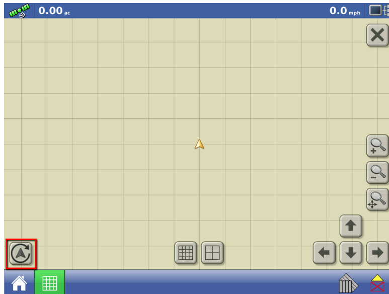
Figure 2 - Press center of map screen and heading change button will appear
